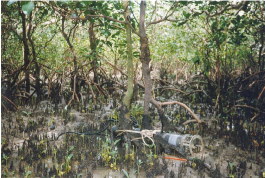
Figure 2.2(b) WHISL SeaPac 2100 wave gauge deployed amongst Rhizophora sp. at the Oonoonba study site. Note red pencil (length ca. 15 cm) for scale.
