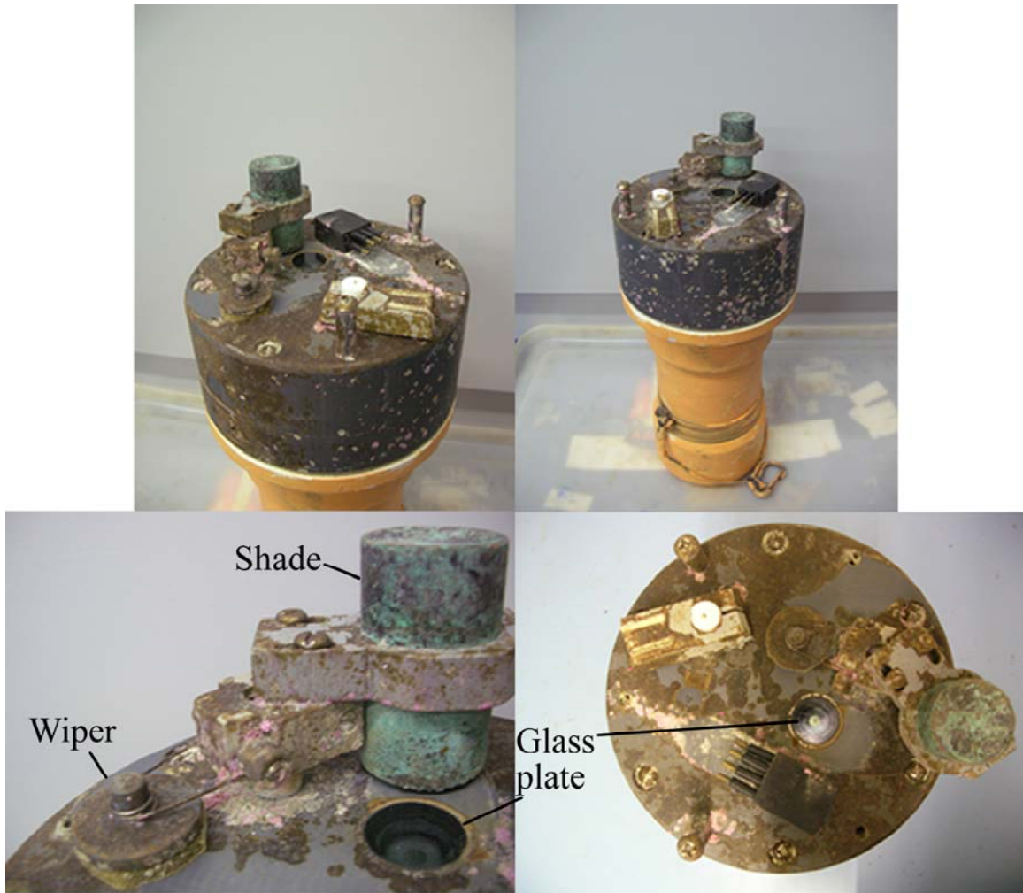
Figure 5.2: Photographs of the Algal Growth Sensor. The circular glass plate, bottom left is the surface on which the algal growth is measured. Behind it is the wiper, bottom left corner of the same picture, and a hollow cylinder, top right corner, which moves over the glass plate to shade it from light during each measurement.
