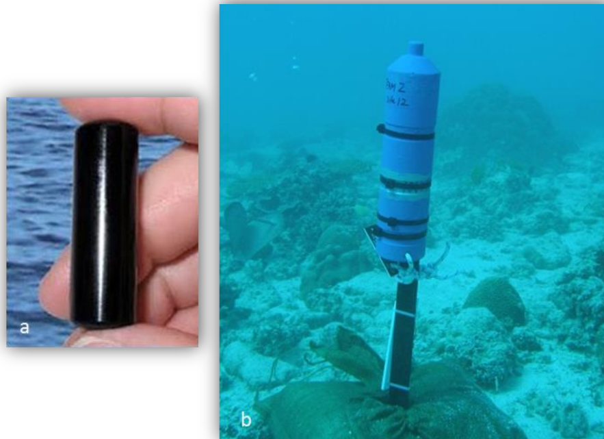
781 782 Figure 3.5 Vemco acoustic telemetry components 783 V13P ® transmitter (a) and the positioning of a VR2W ® acoustic receiver underwater (b) 784 (Photo credits: Vemco Ltd. Canada, A. Boomer). 785
