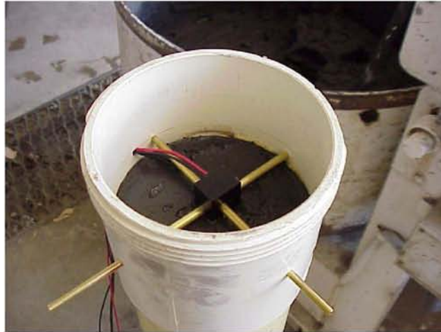
Figure 5.8 – Paste Fill Column Filled to the First Accelerometer
