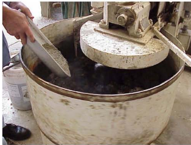
Figure 5.7 – Paste Fill Being Mixed in the Cement Mixer as Cement is Added
