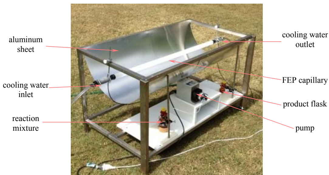
Figure 3.10: Parabolic trough concentrating solar flow reactor.
