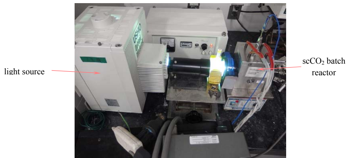
Figure 6.9: Batch reactor for irradiations in \text{scCO}_2 .
