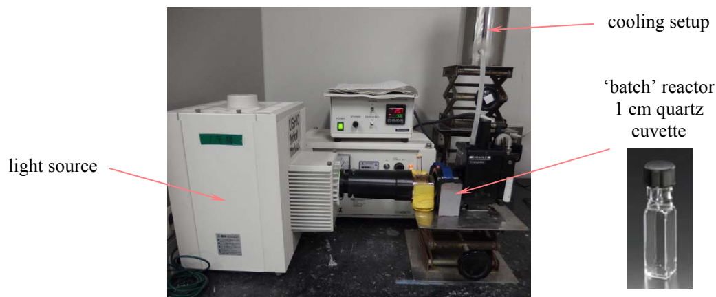
Figure 6.1: Setup for the batch reaction in cyclohexane and cuvette used as a ‘batch’ reactor.
