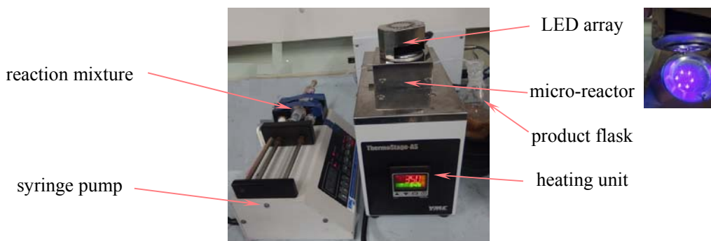
Figure 6.8: YMC keychem-Lumino2 microflow reactor.
